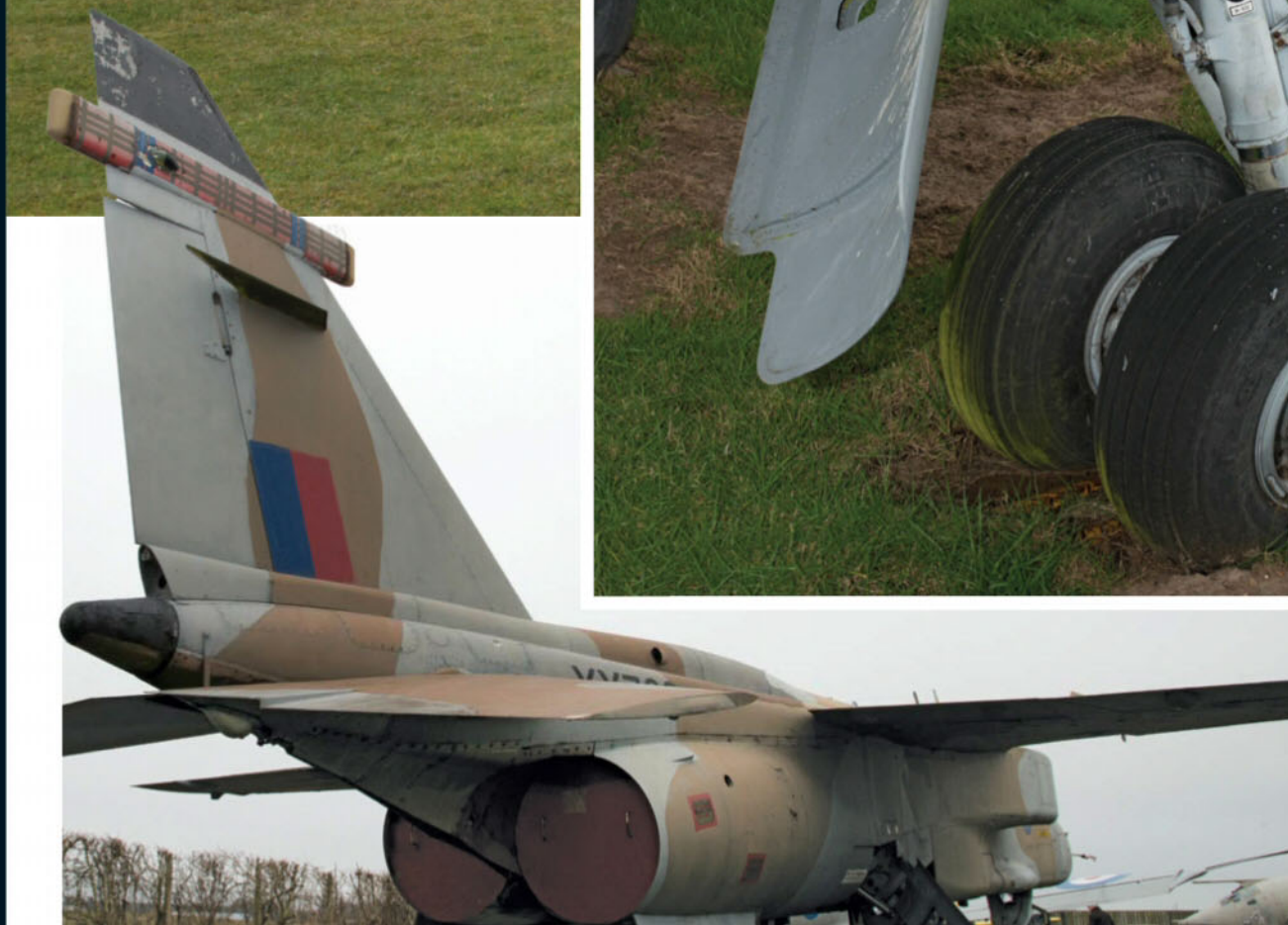
The landing gear's low-pressure tyres retract into the fuselage on takeoff. The IAF initially reported failures, which led to the system being upgraded
